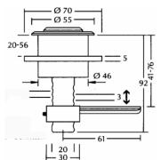
43.964 Hatch fastener with straight cam
