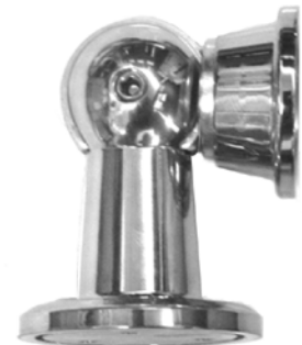
#34.MDH in polished chrome Magnetic door holder Wall or floor or ceiling mounted; For medium weight doors distance: 75.5 mm - 3"high . Brass base material, except for magnet Cup in receiver part galvanized steel.
