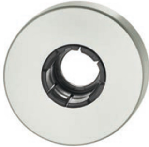
#12.110F.308 Universal rose with inner plastic rose 55 mm diameter. Roses accept all levers and knobs with an 18 mm diameter collar.
