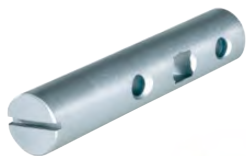
Rose #12.42311 tubular dummy plate with face plate (not shown) use with any lever with 18 mm diameter collar Drill hole 18 mm diameter for 8 x 8 mm spindle
